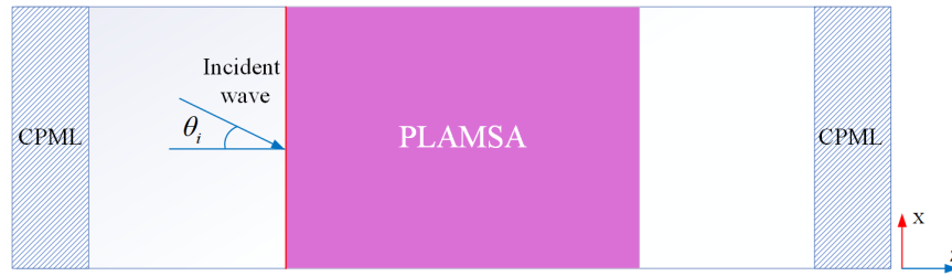
Fig. 1. Schematic of wave propagation in a plasma plate
