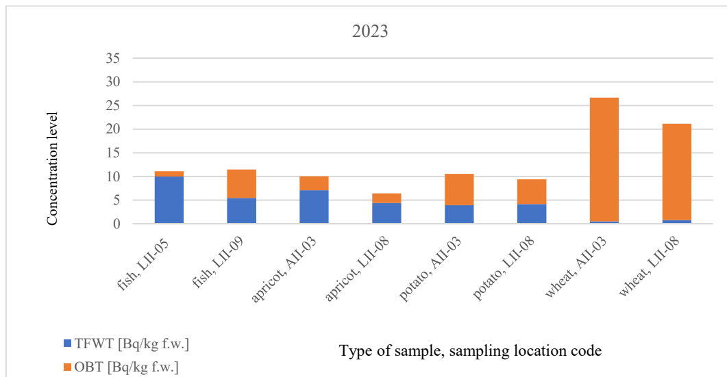
Fig. 8. TFWT and OBT levels in the environmental samples around the Cernavoda NPP, in 2023.
