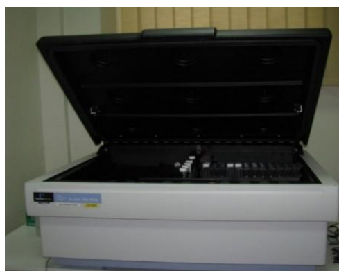
Fig. 4. Sample measurement – LSC, Tri-Carb 3180TR/SL, Perkin-Elmer.
