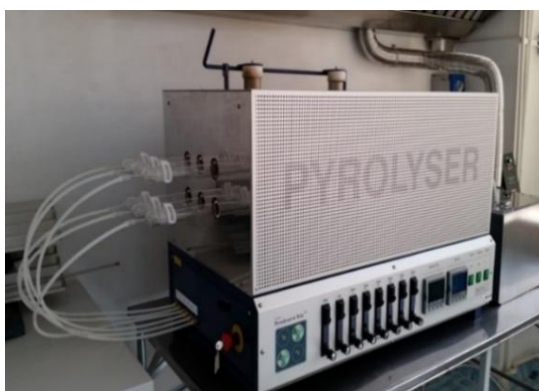
Fig. 3. Sample combustion – Pyrolyser-6 Trio System for ^3\text{H} and ^{14}\text{C} , Raddec.
