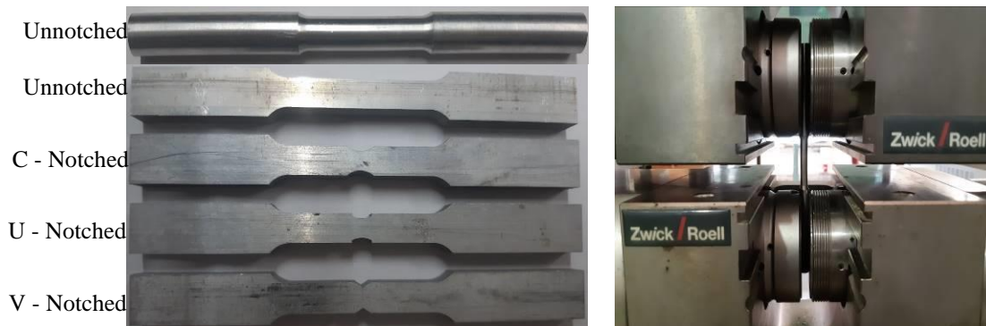
Fig. 1 Tensile tests (a) unnotched and notched specimens and (b) specimens connected between machine crossheads.
