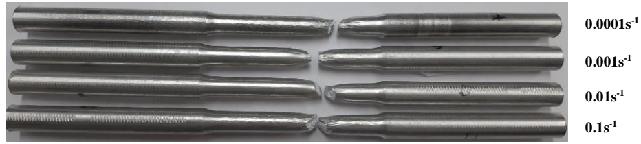
Fig. 3 Broken tensile specimens.
