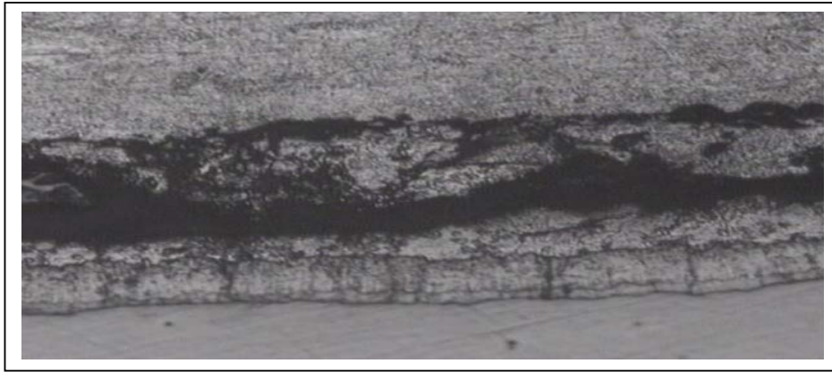
Fig. 7. Optical micrograph (Material COD B) after trying to determine the resistance to stress-corrosion cracking, x 200; ( \text{Na}_2\text{SO}_4 2M , pH =4-5; the value of the applied tension: 74,9 \text{ N/mm}^2 ; the period of time until the sample teared: 56 hours)
