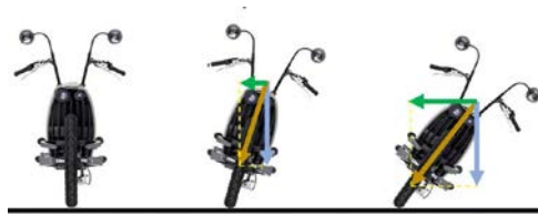
Fig. 3. Forces on steering motorcycle [3]
