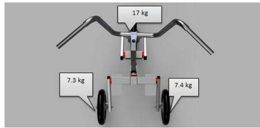
Fig. 10 – The weight distribution of the frame without the user load
