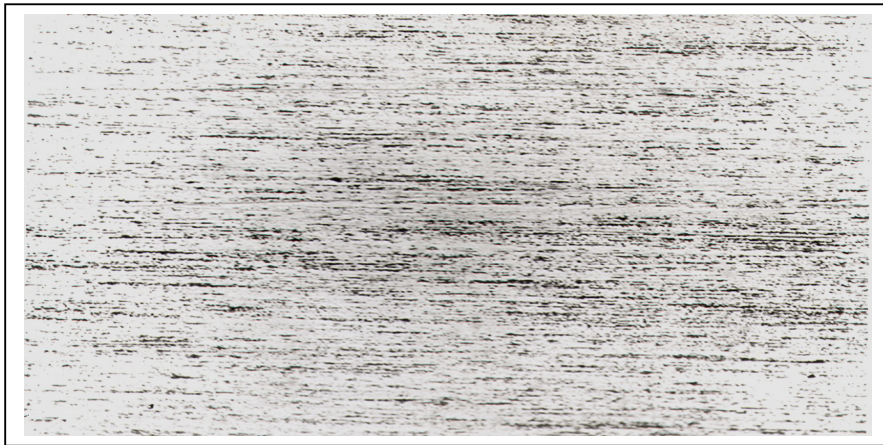
Fig. 6. Optical micrograph of the binary alloy Zn-0.22Cu-0.61Ti (alloy C) in cold rolled condition; x 200; etchant: CrO 3 10%
