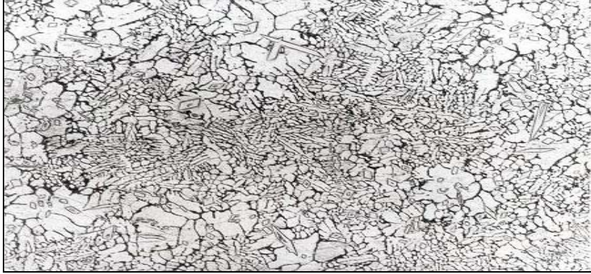
Fig. 2. Optical micrograph of the ternary alloy Zn-0.09Cu-0.19Ti (alloy C) in cast conditions, x 200; etchant: CrO 3 10%
