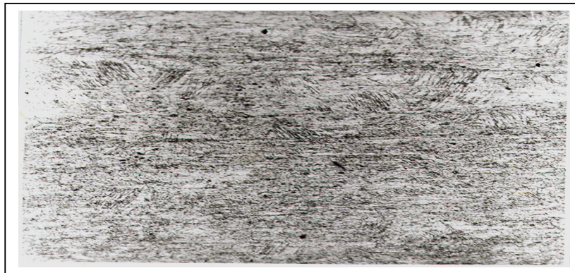
Fig. 4 Optical micrograph of the binary alloy Zn-0,19Cu (alloy B) in cold rolled condition, x 200; etchant: CrO 3 10%
