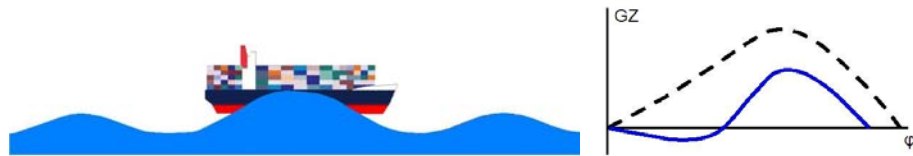
Fig. 4. Large wave is overtaking the ship (left). Decrease of stability caused by the wave crest (right) [12]
