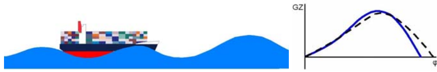
Fig 5. Large wave passed over the ship (left) and the stability is regained (right) [12]
