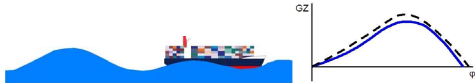
Fig. 3. Vessel sailing in following waves, large wave approaching from stern (left). Changes of stability caused by small relative waves (right) [12]
