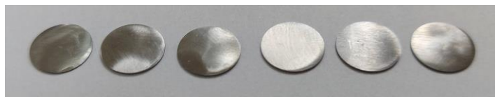
Fig. 4. 316L SPT samples polished with 4000 ppm grit abrasive paper.
