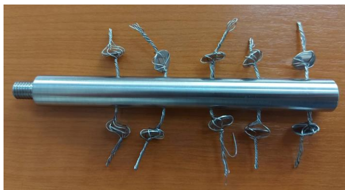
Fig. 5. The 316L sample holder for pre-exposure in liquid lead environment.
