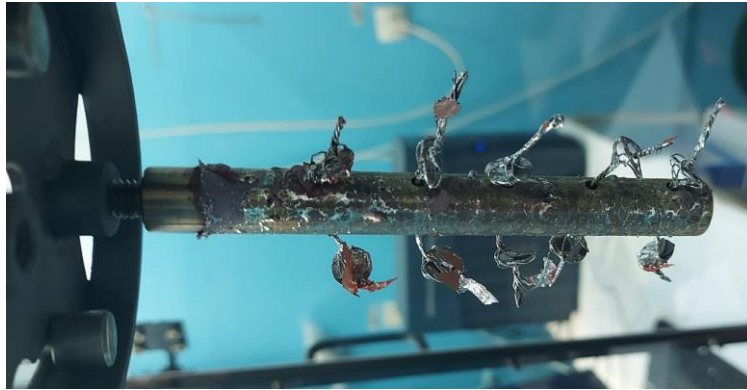
Fig. 6. SPT samples after exposure to molten lead environment.
