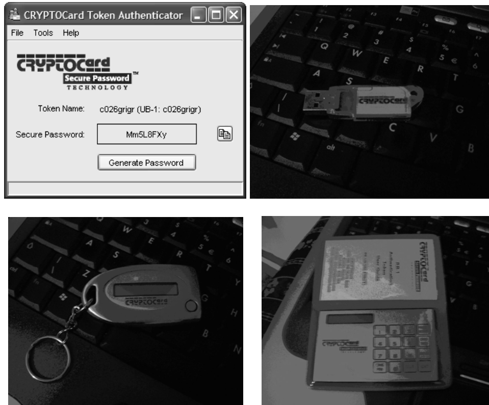
Fig.3. Three types of OTP tokens. USB/software version, key-chain and calculator versions.
