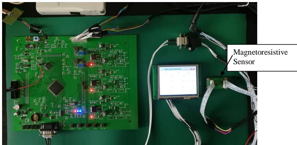
Fig. 9. Diagram of the circuit board of the measuring device of AC and DC weak MFD.
