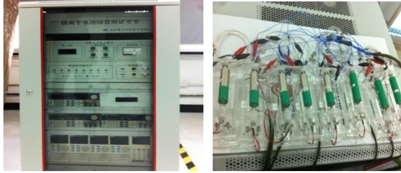
(a) NCA/C spaceborne lithium battery (b) comprehensive test equipment of satellite lithium battery Fig.3 satellite lithium battery and experiment equipment.
