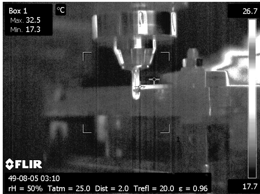
Fig. 2. Temperature variance into the cutting zone
