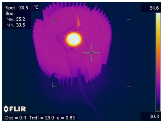
Fig.29. Temperature on the heat sink after 60 minutes for the fitting with the synthetic air jet generator
