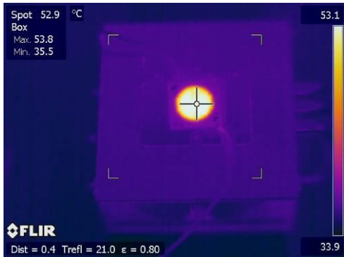
Fig.16. Measurement results after 90 minutes for the lighting fitting with the fan turned on
