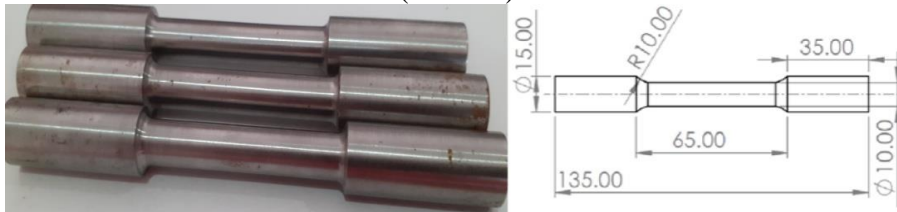
Fig. 2. The conventional specimen shape and dimensions according to the ASTM E466-07 standard
